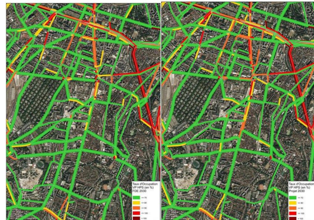
FIGURE 21 : NIVEAUX DE SATURATION A L'HPS 2030 SCENARIO FDL (ILLUSTRATION DE GAUCHE) ET SITUATION DE PROJET 2030 (ILLUSTRATION DE DROITE)
